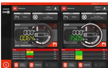
Displaying 2 transducer readings simultaneously
