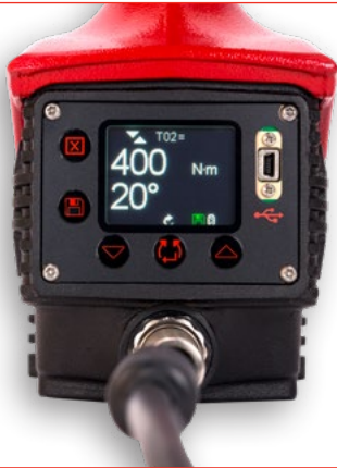
Colour OLED display shows torque and angle values
