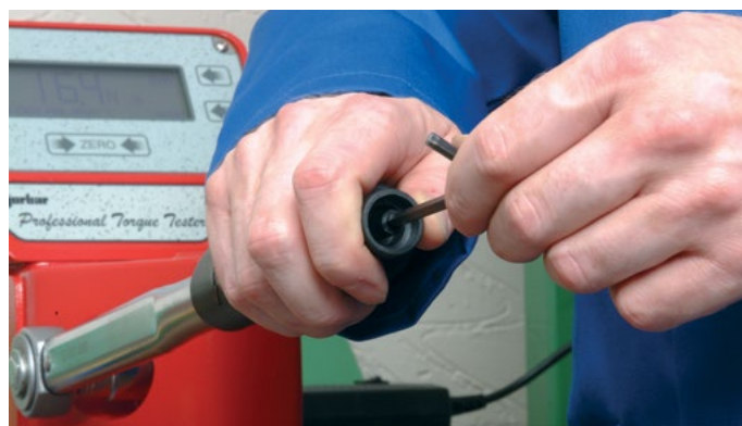
Setting a 'P' Type Torque Wrench
