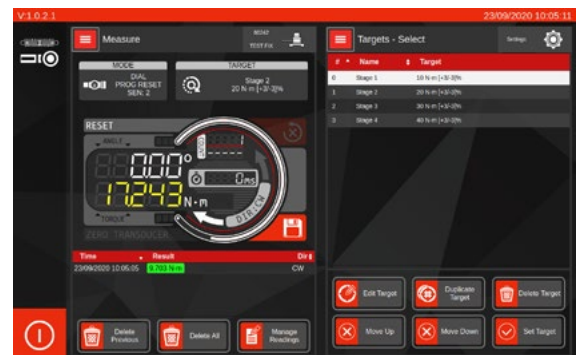
Displaying transducer reading alongside target selection
