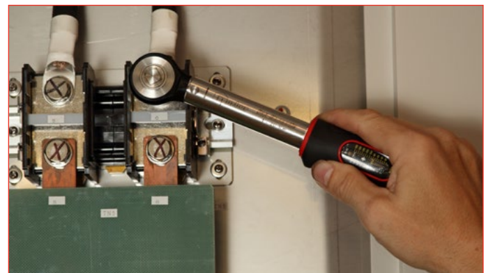
TTi20 Non-Magnetic in application on an MRI Scanner
