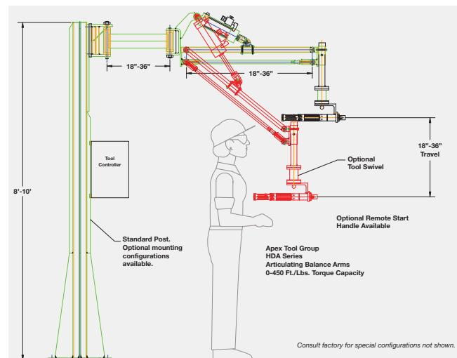
structural column, ceiling mounted or post. The tool is typically mounted on the end of the arm.
