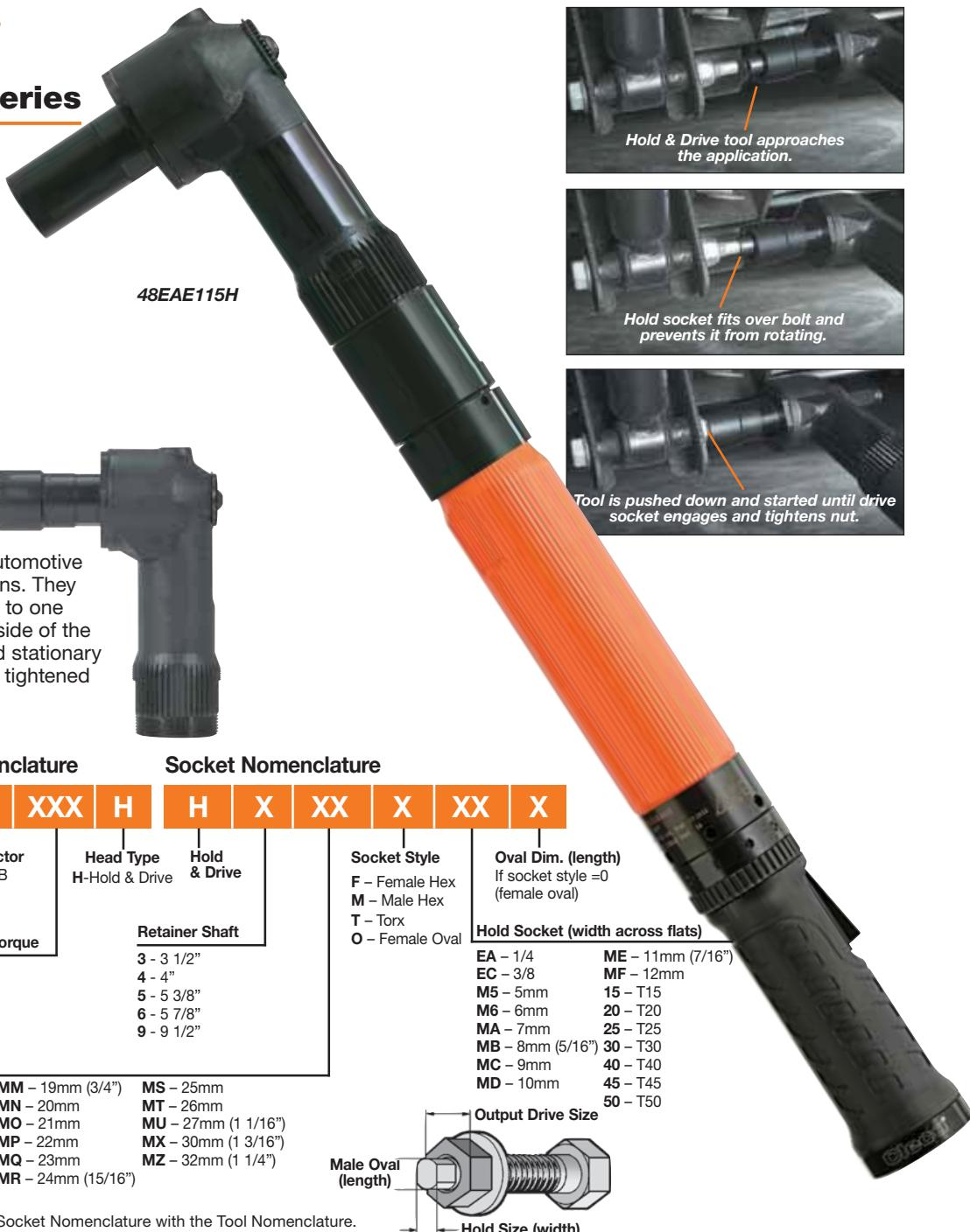
"Hold & Drive" bolts are used with these tools in automotive and truck frame applications. They reduce assembly handling to one person working from one side of the workpiece. The bolt is held stationary by the tool while the nut is tightened from the same side.
