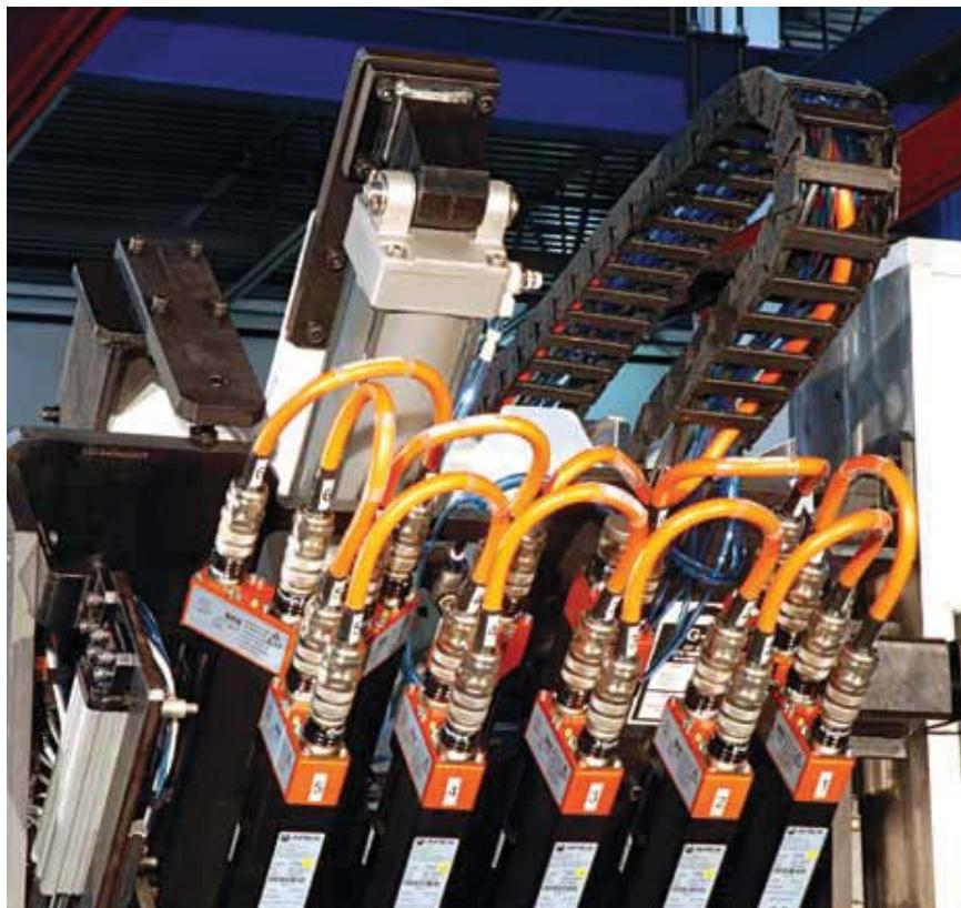
*Shown above is a ten Intelligent spindle application with nine jumper cables and a single field cable that terminates at the power distribution box.*
