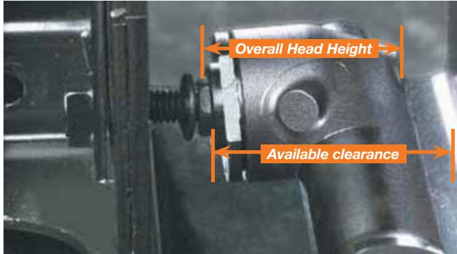
Flush socket tools have plenty of clearance to fit low clearance applications. Electric flush socket tools tighten with much higher accuracy than tools with crowfoot attachment.
