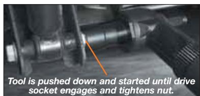
"Hold & Drive" bolts are used with these tools in automotive and truck frame applications. They reduce assembly handling to one person working from one side of the workpiece. The bolt is held stationary by the tool while the nut is tightened from the same side.
